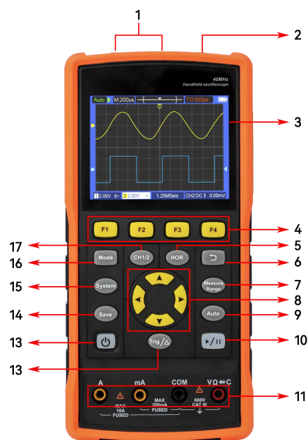
Figure 4: Front Panel of the Oscilloscope
