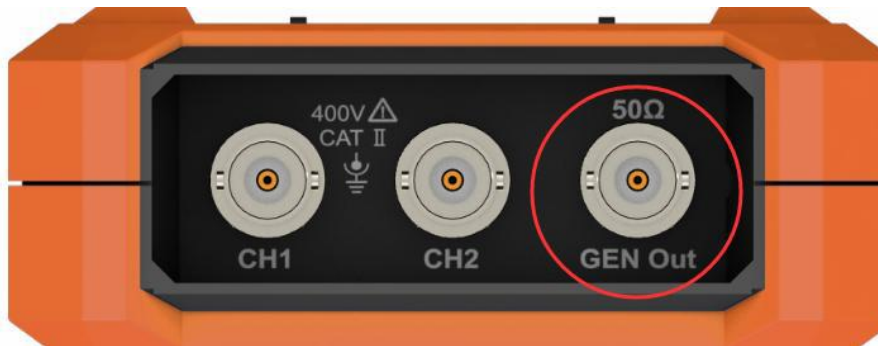
Figure 5- 1: Generator Output Ports
