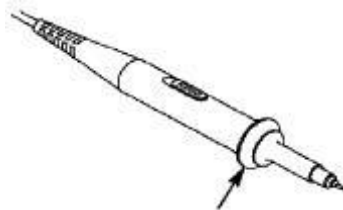
Figure 0-5: Finger Safety Ring of the Probe
