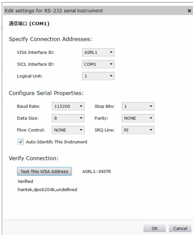
The IO software "My instrument" COM list shows the connected devices, click "interactive IO", and send any command, the computer and the device get communication.
